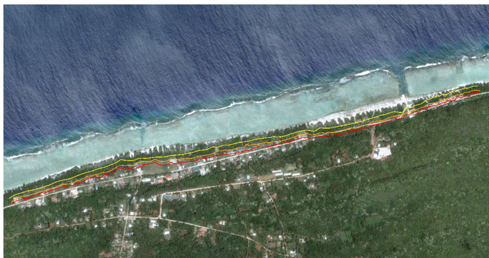
Figure 23. Draft 10, 50 and 100 year ARI cyclone run-up levels derived for the Oneroa village frontage. The 10 year ARI run-up level is shown in yellow, the 50 year ARI in orange and the 100 year ARI in red. The run-up levels were produced by version 1.17 of the Cook Islands Coastal Calculator which has subsequently been updated.
