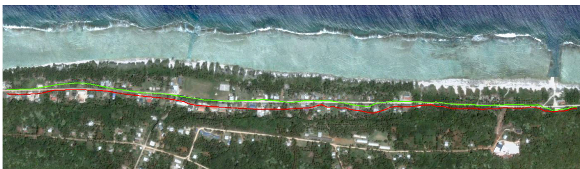
Figure 31. Final cyclone hazard lines developed for the 2030s and 2060s for Oneroa village, Mangaia, Cook Islands. The lines indicate a possible chance of wave run-up due to a 50 year ARI cyclone event reaching this level over the period from the present to the 2030s (green line) and a possible chance of wave run-up due to a 100 year ARI cyclone event reaching this level over the period from the present to the 2060s (red line).
