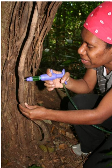
Emily Tasale (EDA) using dyed water to test an injector fitted with a blind needle. These will be used to inject undiluted glyphosate (Weedmaster) into large stems.
